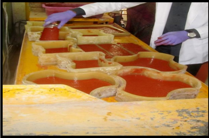
Casting of paver blocks
