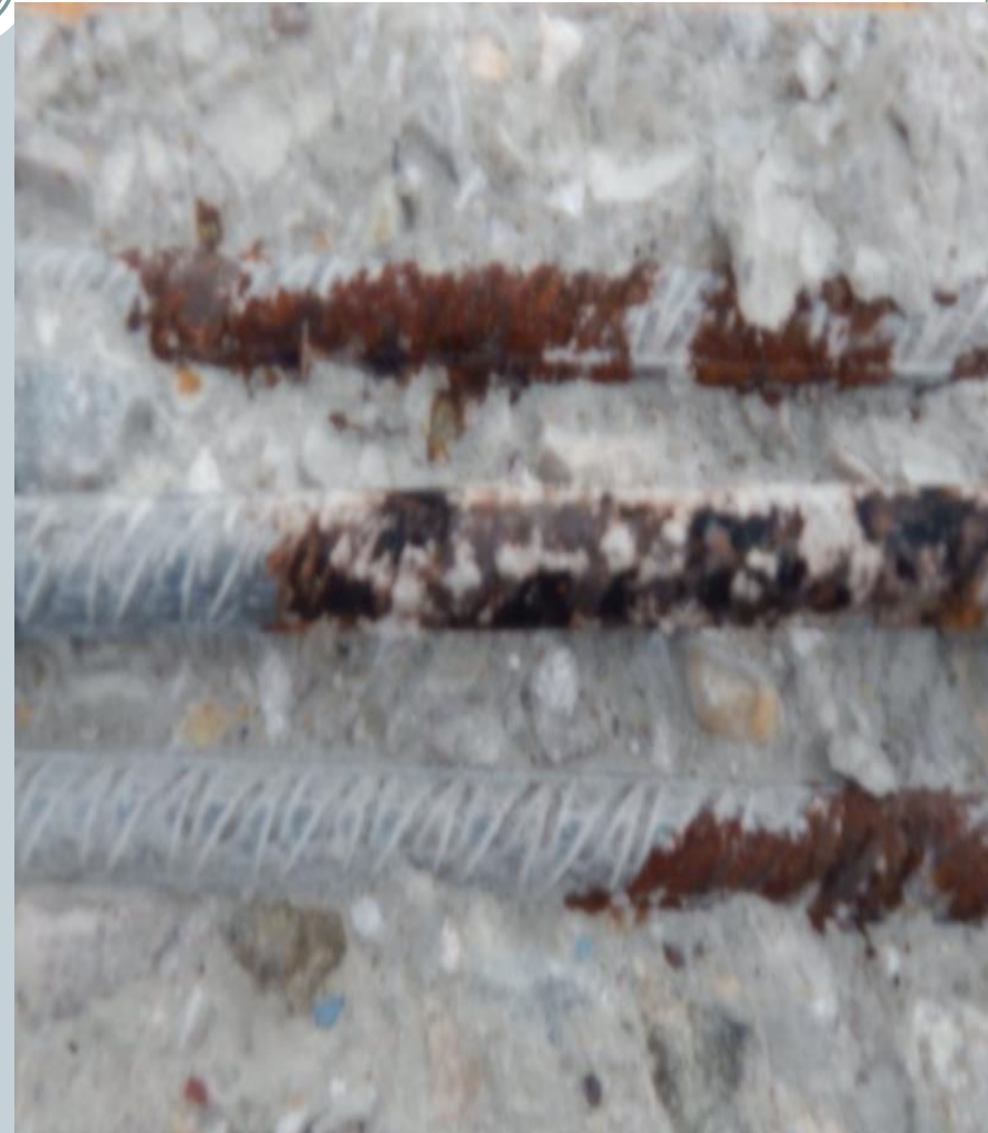
Broken corrosion specimen for visual examination
